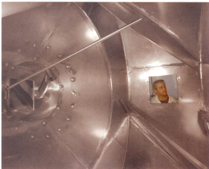
ABOVE: Rotating drum with proprietary mixing flights achieves total batch uniformity in less than three minutes
